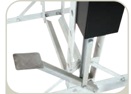
Foot Pedal For Hydraulic Pump HPF-20 Shown
