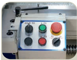
Saddle Switch Board
