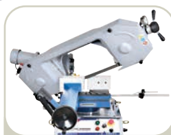
Head Swivel to 60 Degrees EB-285DSV
