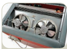
Thermostatically controlled cooling fans (K30SI & K50SI)
