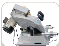
Compound Cut at 45 Degrees Left View
