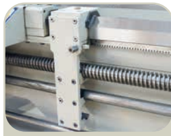
Leadscrew and Feedscrew Support Recovered
