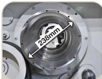
Large 238mm Spindle Bore
