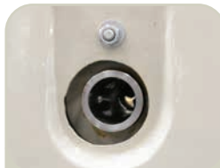
40mm Spindle Bore AL-960B
